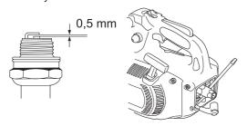
Note! Always use the recommended spark plug type! Use of the wrong spark plug can damage the piston/cylinder. Check that the spark plug is fitted with a suppressor.
